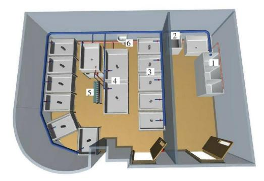
Fig. - Scheme of the mini-RS equipment in the lab room
